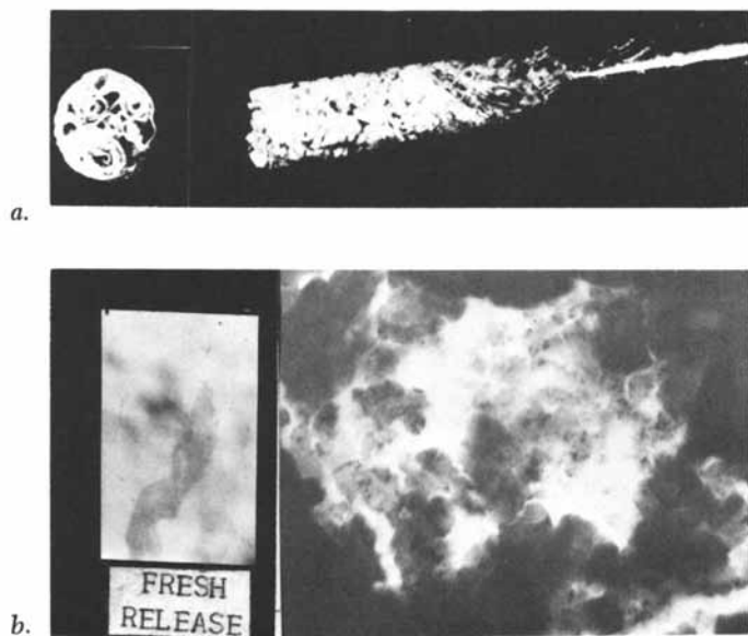
Figure 6. Crown polystyrene of 1949: (a) whole sample, and in cross-section; (b) electron micrograph (100,000 \times ), with inset (450 \times )
